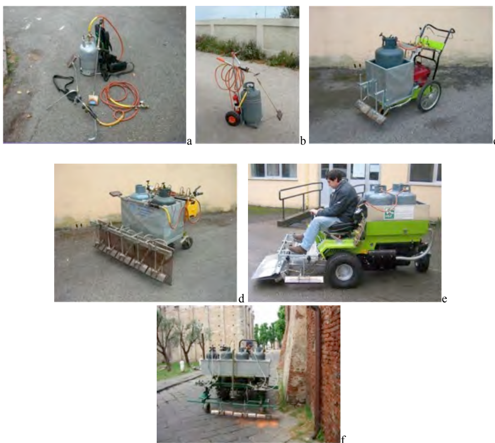
Figure 5. Pictures of innovative machines for flame weeding working in urban areas: a) knapsack machine; b) trolley machine; c) trimmer machine; d) wheel barrow machines; e) rider machine; f) mounted machine.
