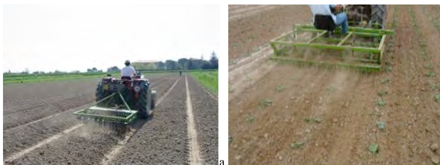
Figure 2. First version of rolling harrow during a full-width intervention before spinach sowing (a) and second version, equipped with guidance system and elastic tines for in-row weed control, during an hoeing treatment on cabbage.
