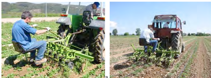
Figure 4. (a) Precision hoeing for narrow inter-row spaces during a post-emergence intervention on spinach; (b) precision hoeing for wide inter-row spaces during a post-transplanting intervention on processing tomato.
