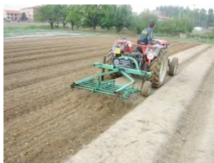
Figure 1. (a) Diagram of the spring-tine harrow: (A) main frame; (B) supporting wheel; (C) U-shaped support; (D) modular secondary frame; (E) tine slope regulation lever; (F) chains; (G) spring tines. Detail: (d) working direction; (a) = 25 cm (b) 11 cm; \varnothing = 6 mm; a = 135^\circ ; b = 45^\circ ; g = 15^\circ ; (b) spring-tine harrow at work before spinach sowing.
